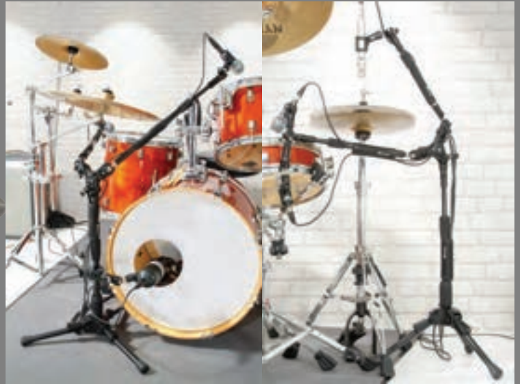
Components used on these systems: (1,3&6) O2 or O2X Dual booms. (2) T3 Stand. (4,5) T1 stands. (7) IO-Vector. (8) IO-C or IO-GCM. (9) All mic positions use M2 adapters.
