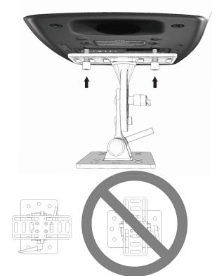
DO NOT mount the SM-UM1 horizontally. To mount your speaker(s) vertically or horizontally, use the four (4) faceplate machine screws to fasten the faceplate to the desired speaker position.
