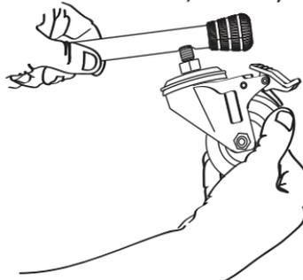
On the underside of each leg (just behind the foot) you will find the head of the stainless steel connector bolts. The casters are attached to the T3 legs with these bolts. Removed the connector bolts with the included 8mm hex wrench. Once the bolts are removed you are ready to install the casters.
