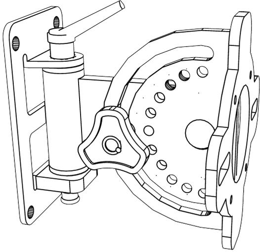
The SM-SW1 is the main pan and tilt swivel for the SM-1 System. The SM-SW1 controls are redundant with both a locking spring pin and tension knobs. The set position holes are set in 15° increments.
