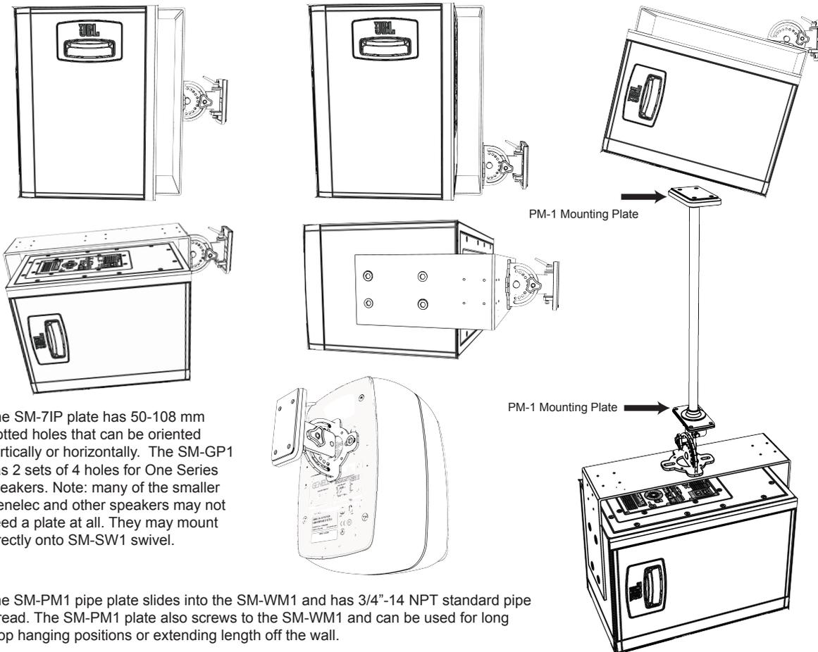
The SM-7IP plate has 50-108 mm slotted holes that can be oriented vertically or horizontally. The SM-GP1 has 2 sets of 4 holes for One Series speakers. Note: many of the smaller Genelec and other speakers may not need a plate at all. They may mount directly onto SM-SW1 swivel.
