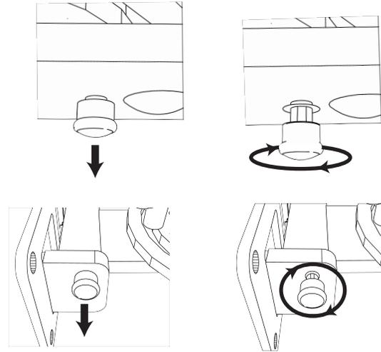
While pulling out turn the knob 90° and release it. It will stay locked out in this position. Move the swivel to the desired position and to lock the pin in, pull and turn 90° again and it will find the nearest hole. You can also pull the pin and not turn it, move the swivel and let it lock in the the next hole with the spring.
