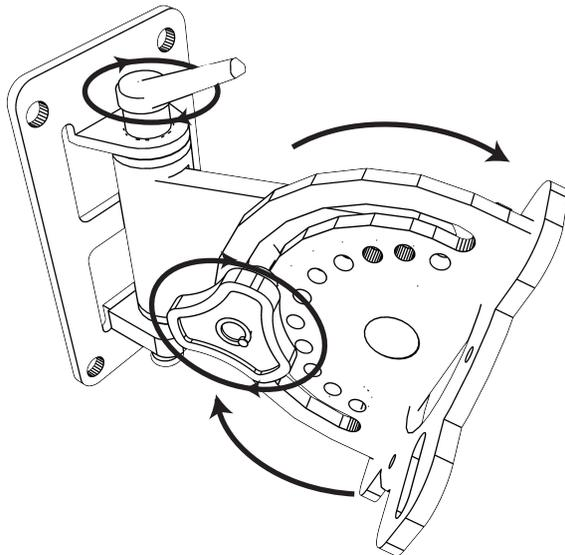
To adjust them, first loosen the tension knob and then pull the spring pin out.
