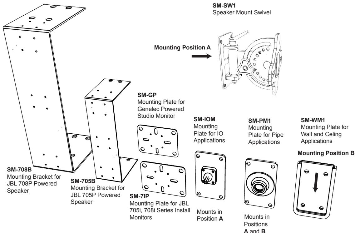
The SM-1 Atmos Mounting System offers the installer many options for mounting on walls, ceilings or Triad-Orbit IO®.
