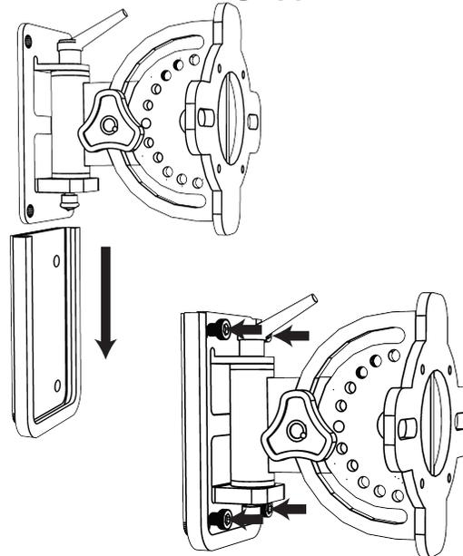
The SM-WM1 wall pate should be mounted in position prior to loading. This allows for installers to preset all the speaker positions before seeing the speaker up. The SM-SW1 then slides into the SM-WM1. Use the provided hex screws to secure it into the wall plate.
